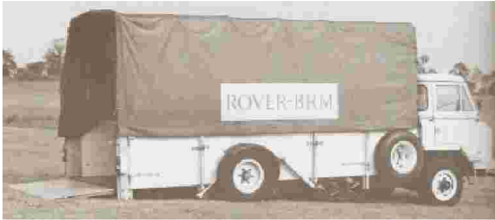
This “kneeling” truck was developed to transport the Rover-BRM to Le Mans in 1965. It was front wheel drive only.
